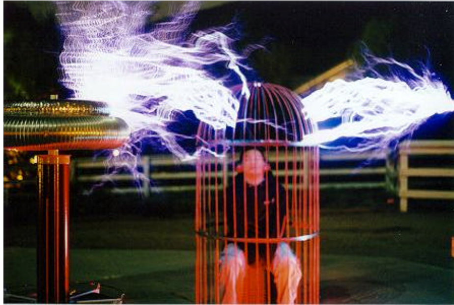
Live demonstration of a Faraday Cage. The electricity travels on the outside.
