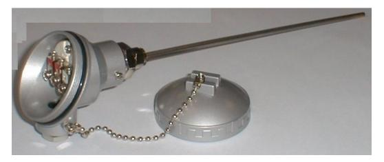
These rigid sensors have a stainless steel welded closed end sheath. The Pt100 sensing element is 10mm long and is placed at the tip of the sheath which means that the minimum immersion depth should be at least 50mm. The sensor is rated up to 350°C. They are terminated with an IP67 standard weatherproof head. Ideal where a heavy duty connection needs to made near to the sensor.
